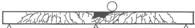
d) 移動繰返し載荷実験(せん断破壊): M10-75, No. 19 (P=5.0tf, N=8038)
