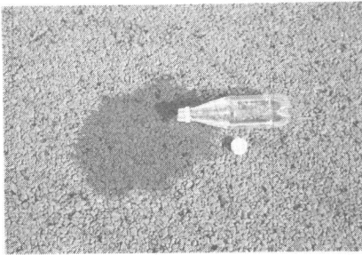
Photo 1 Water percolates quickly into "no-fines" previous concrete
