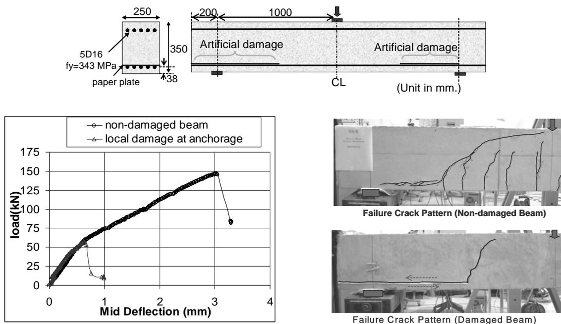
Figure 7 Load-deflection and failure mode of anchorage zone damaged beam – Case (4) -
