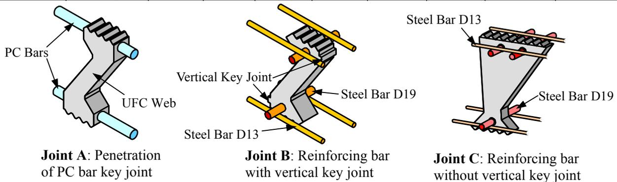
**Fig. 1 Three types of joint method**
