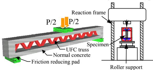
**Fig. 2 Flexure-shear test of composite beams**
