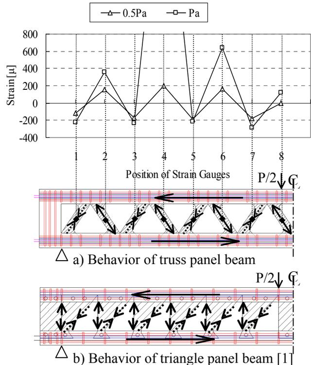
**Fig. 6** Behavior of composite PC beams by applying UFC as perforated web member
