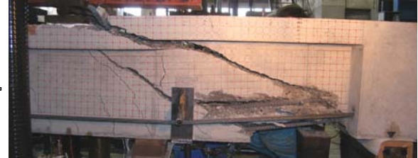
(b) Crack Patterns for ns14 (Right-half of the beam)
