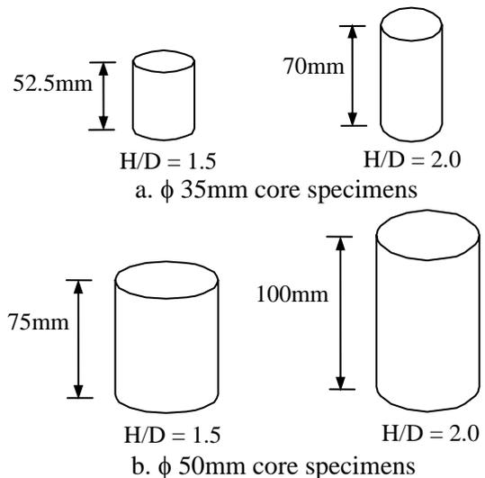
Figure 7 Core cylinder specimens
