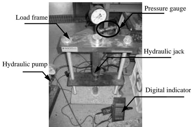
Figure 4 Point loading test devices
