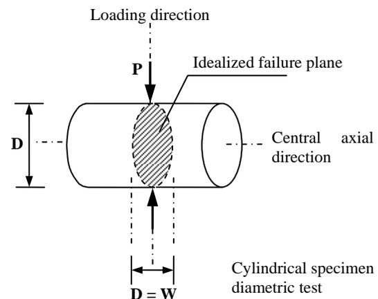
Figure 1 Specimen dimensions for a diametric point load test on cores
