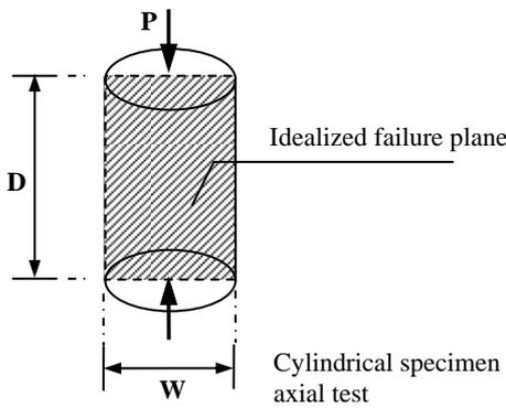
Figure 2 Specimen dimensions for an axial point load test on cores
