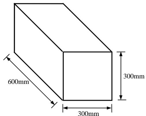
Figure 3 Dimension of block specimen
