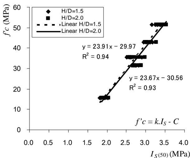
Figure 11 Correlation graph for point load strength index to compressive strength
