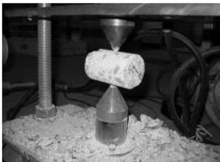
Figure 5 Point loading test situation
