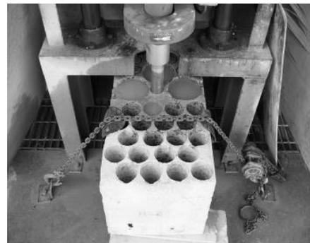
Figure 6 Core cylinder extractions
