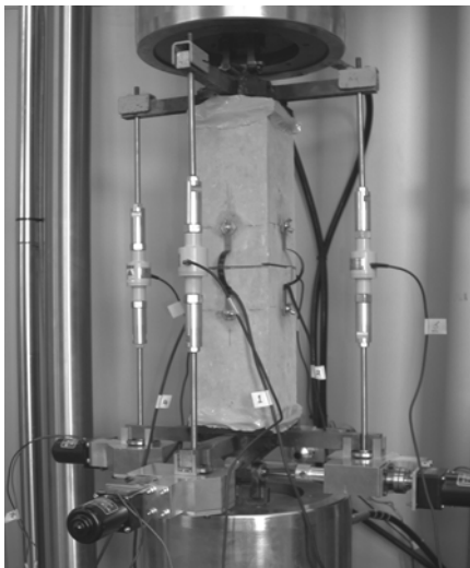
Fig. 1 Adjusting gear system and experimental set up
