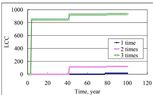
Fig.8 Life cycle cost based on using actual inspection result
