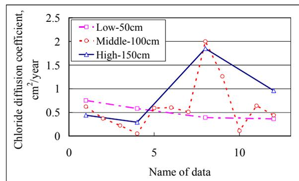
Fig.6 Effect of height from sea water level on chloride diffusion coefficient
