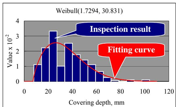
Fig.4 Distribution fitting of the inspection result
