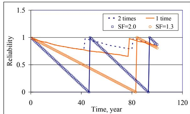
Fig.9 Reliability of structure along service life
