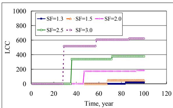
Fig.7 Life cycle cost based on using safety factor
