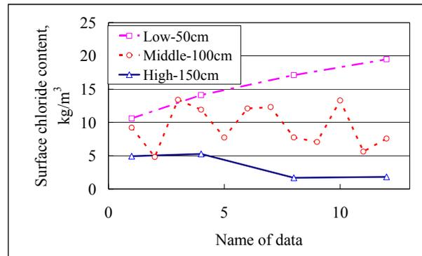
Fig.5 Effect of height from sea water level on surface chloride content
