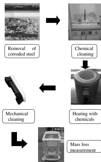
Fig.6 Gravimetric mass loss determination
