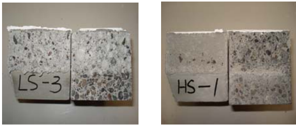
(a) LS series (b) HS series PHOTO 1. Fracture of interface
