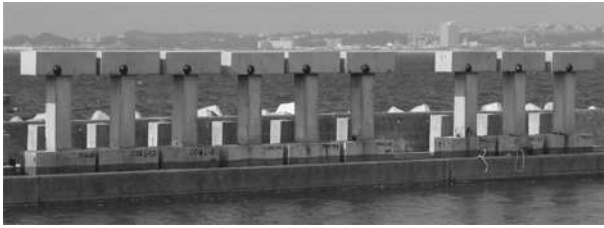
Photo 1 Exposure of RC column specimens in Okinawa seashore.
