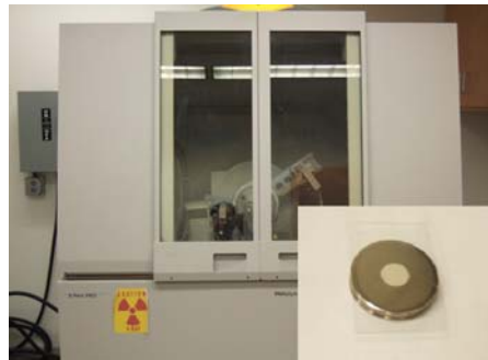
Fig. 3 Test machine and sample for XRD analysis
