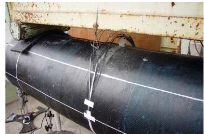
写真-3 CFS 破断 (D4F9P14L2T1FC)
