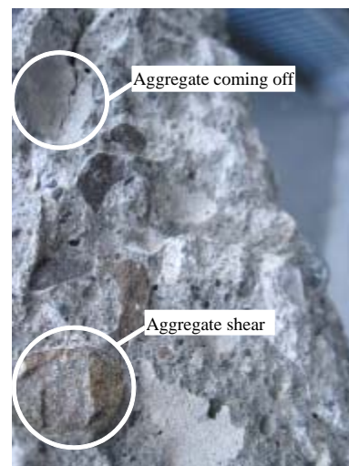
Fig. 2 Failure plane of recycled aggregate concrete
