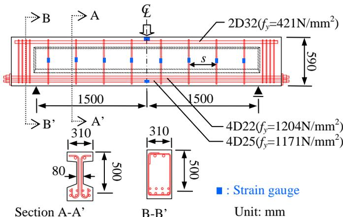
Fig. 1 Dimensions and steel layout of specimens
