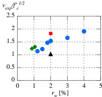
Fig. 9 Effect of stirrup ratio ( $r_w$ )
