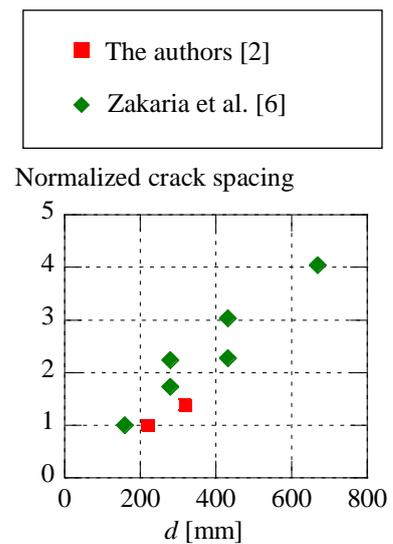
Fig. 8 Effect of  $d$  on diagonal crack spacing
