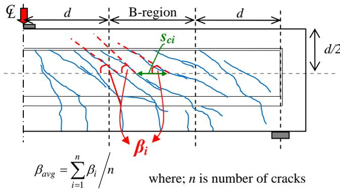
Fig. 3 Example of crack spacing and angle measurement
