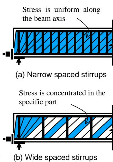
Fig. 7 Effect of spacing of stirrups
