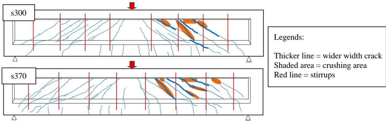
Fig. 5 Crack patterns just before the peak load
