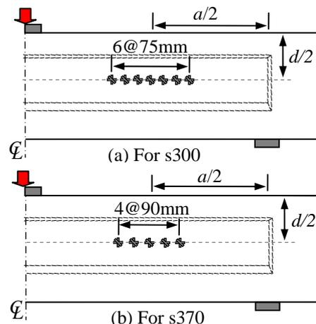
Fig. 2 Location of tri-axis strain gauges
