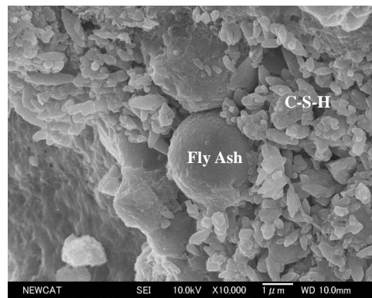
Photo 5 SEM Photo of [3h Steam(80°C) Cured] Non-Burnt Brick Specimen (FA: India-B) (×10000)
