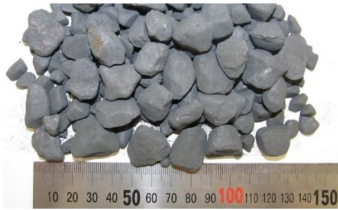
Photo 1 High-Density Aggregate( \mu = 4.5\text{g/cm}^3 )
