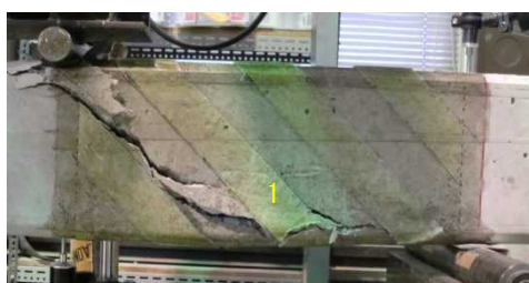
写真-10 No. 10 (50% 135度) せん断破壊
