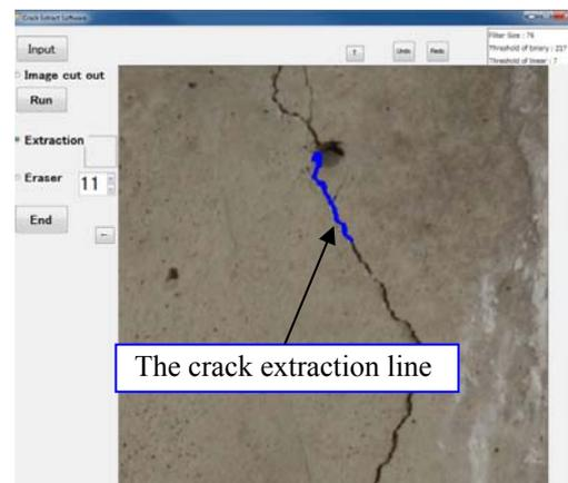
Fig.10 Crack extraction image
