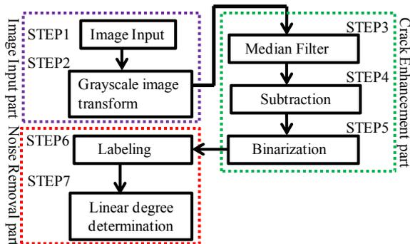
Fig.3 Image processing technique
