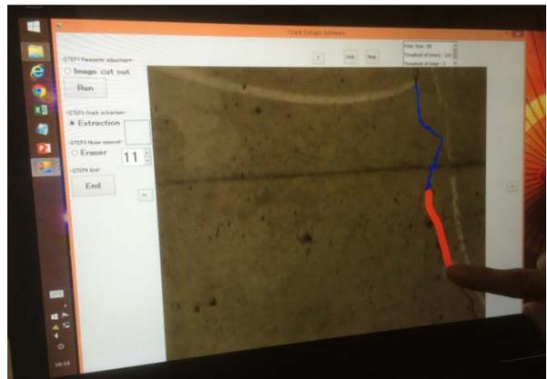
Fig.1 Touch screen for detecting crack by finger tracing
