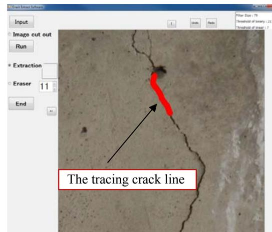
Fig.9 Tracing crack on background image
