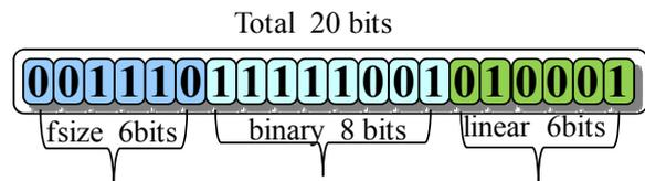
Fig.5 Coding presentation of a solution candidate
