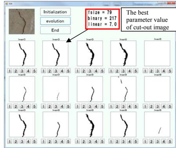
Fig.7 Parameter adjustment window
