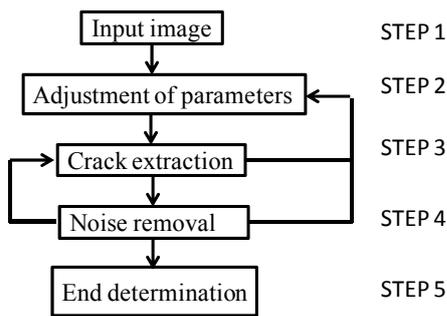
Fig.2 Operation procedure of the software
