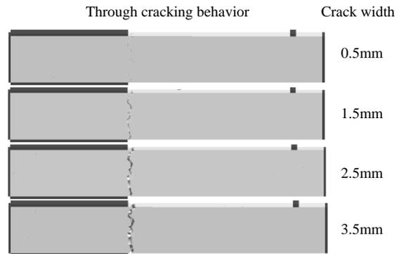
Fig. 10 Through cracks by tension of link elements (case 1)
