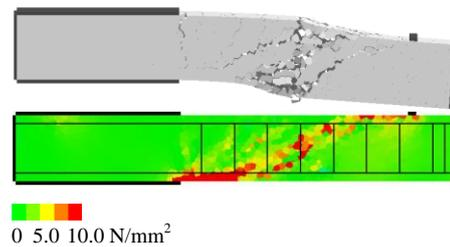
Fig. 16 Deformation behavior and principal stress distribution in column central section (Peak load, crack width of 3.5mm of case 3)
