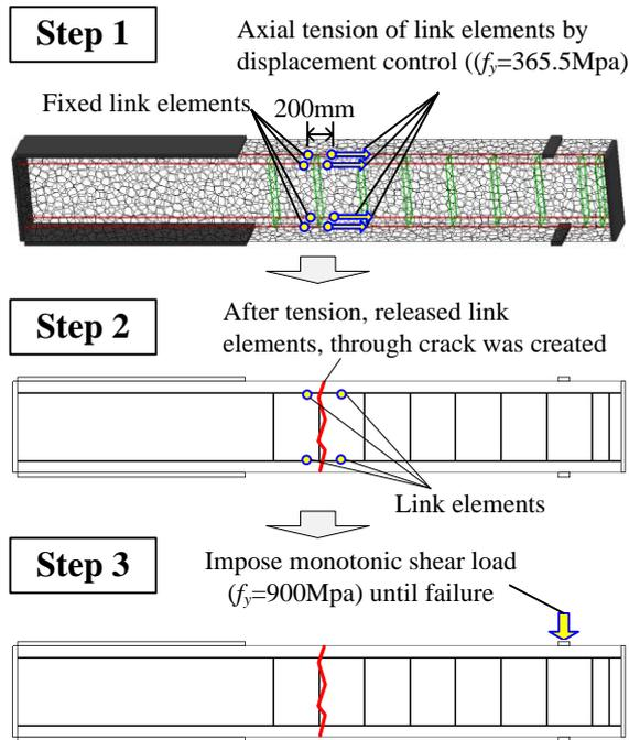
Fig. 9 Evaluation method of shear strength after creating initial through crack
