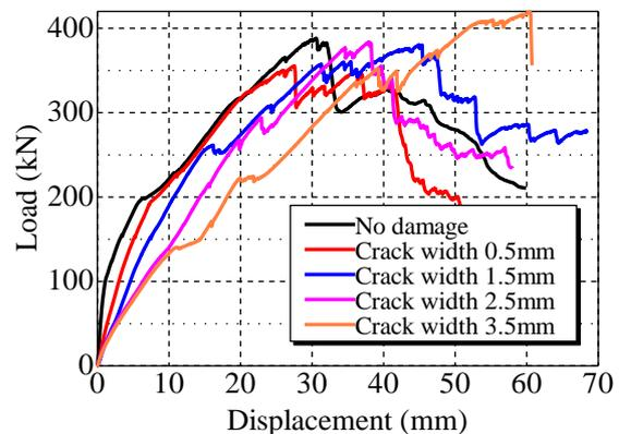
Fig. 11 Shear load-displacement relations (case 1)
