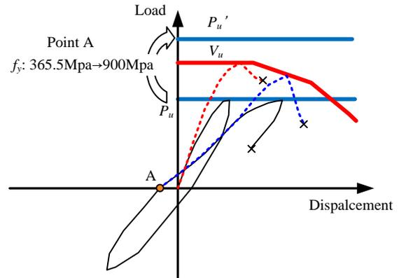
Fig. 6 Evaluation method of shear strength degradation due to cyclic loading
