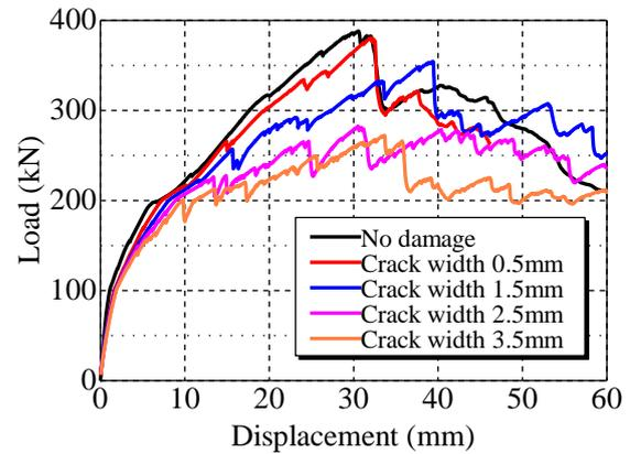
Fig. 15 Shear load-displacement relations (case 3)
