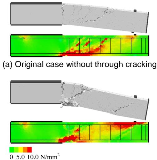
(b) Through crack width of 3.5mm (case 1)
