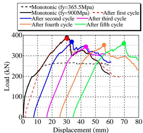
Fig. 8 Load-displacement relations for evaluation of degraded shear strengths after each load cycle of one-side repeated loading
