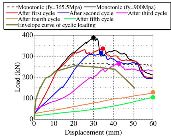
Fig. 7 Load-displacement relations for evaluation of degraded shear strengths after each load cycle of cyclic loading
