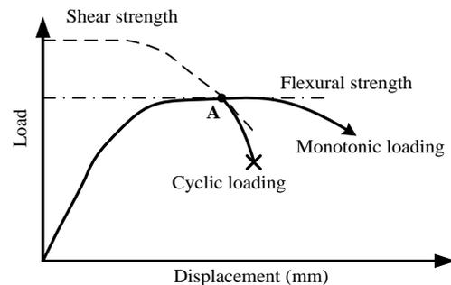
Fig.1 Reason of shear failure after flexural yielding
