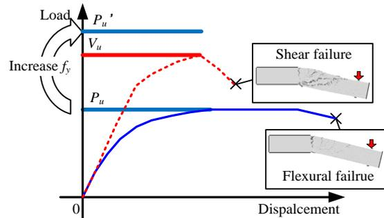
Fig. 4 Evaluation method of shear strength of flexural yield type RC member
