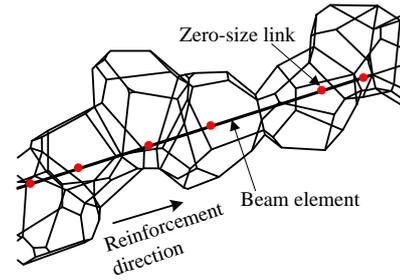
Fig. 3 Reinforcing bar model
