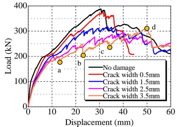
Fig. 13 Shear load-displacement relations (case 2)
