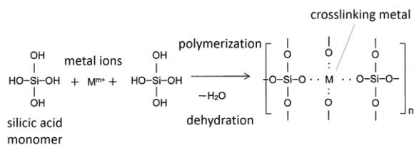
Fig. 1 Crosslinking and polycondensation [4]
