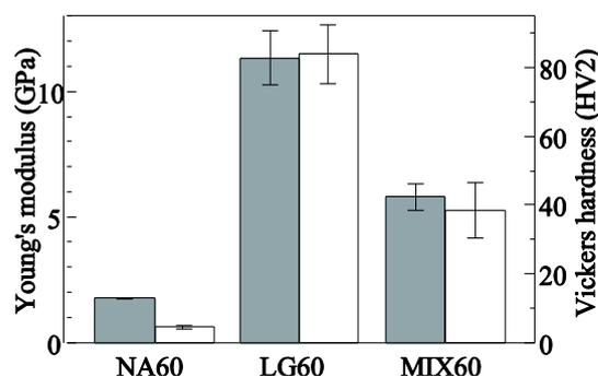
Fig. 7 Young's modulus and Vickers hardness by indentation test
