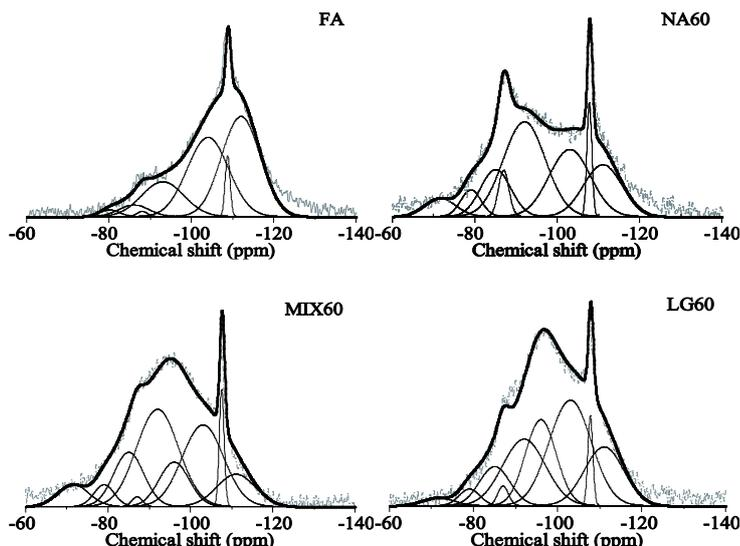
Fig. 5 Deconvolution of NMR signals for FA, NA60, LG60, and MIX60. The samples were cured for 24 hours.
