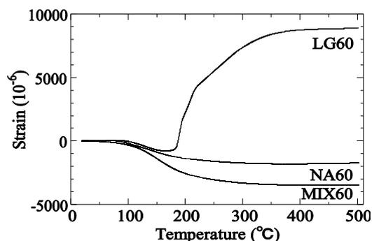
Fig. 8 Expansion / contraction as temperature increase
