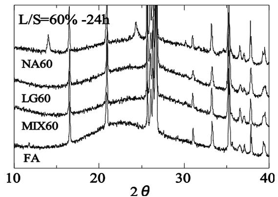
Fig. 3 Variation of the halo peak to the high angle
