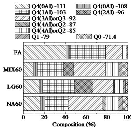
Fig. 6 Relative composition ratios of the  $^{29}\text{Si}$ -NMR peak intensity
