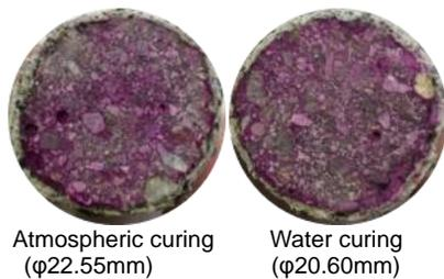
Fig.8 Neutralization depth indication for OPC
