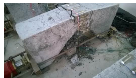
(a) Specimen without corrosion (F0)
