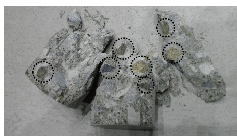
Fig. 1 Fracture condition of G2 aggregate[1]
