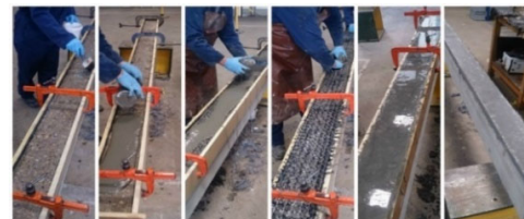
Fig.2 Preparation of TRM strengthening layer
