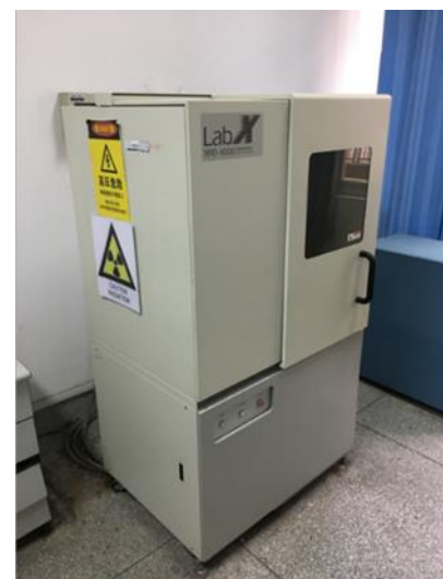
Fig.3 XRD-6000 model X-ray powder diffractometer
