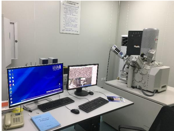
Fig.4 Nova NanoSEM450 scanning electron microscope (SEM)
