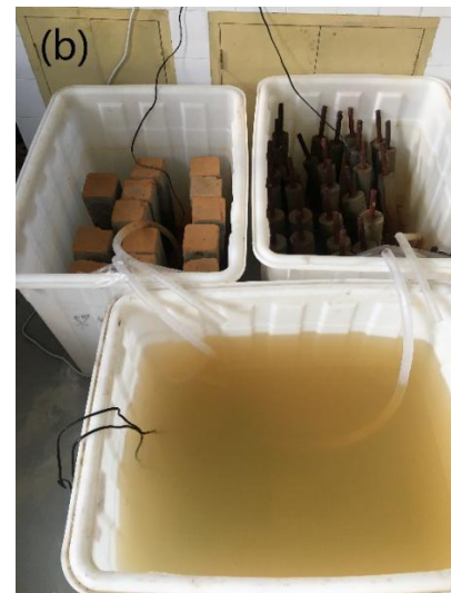
Fig.2 Accelerated corrosion test; (a) Immersion, (b) Wet/dry cycles
