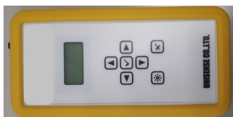
(c) Digital penetration depth measuring device
