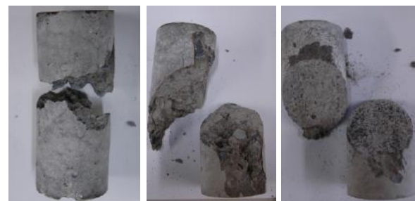
(a) 0.5h C (b) 1.0h CS (c) 3.0h S C : Compression S : Shear CS : Compression + Shear
