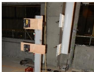
Fig.3 Building instrumentation; (a) accelerometers, (b) laser transducers, and (c) potentiometers
