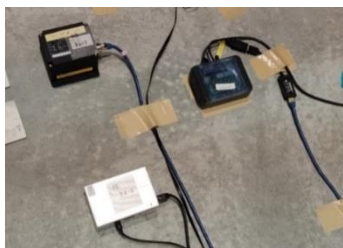
Fig.3 Building instrumentation; (a) accelerometers, (b) laser transducers, and (c) potentiometers
