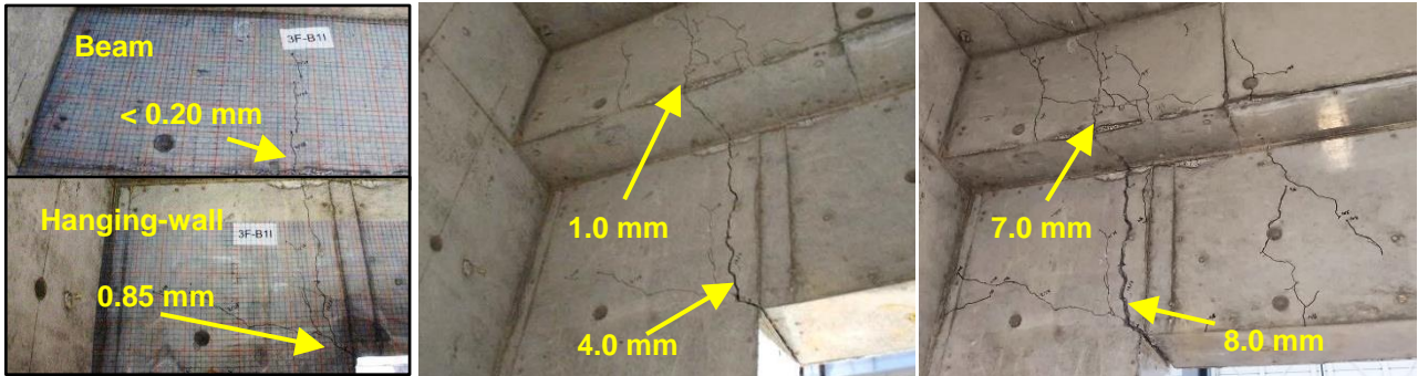
(a) After 1.0-scaled (b) After 1.5-scaled (first run) (c) After 1.6-scaled Fig.7 Progression of damage in 3F-B1 beam-wing wall joint (residual widths of largest crack indicated)
