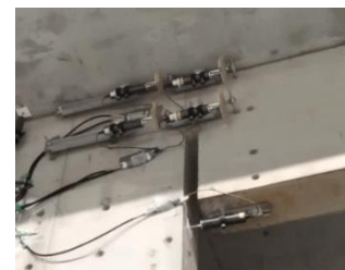
Fig.3 Building instrumentation; (a) accelerometers, (b) laser transducers, and (c) potentiometers
