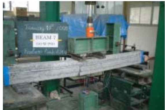
Fig. 4 Failure of beam B7 (G0 -W- P60)
