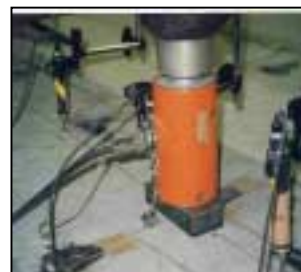
Fig. 2(e). Loading cell with the loading pad
