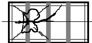
Fig.4b. Control specimen bottom cracks during A1 loading
