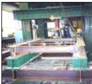
Fig. 2(c). Overall support frame for main frame
