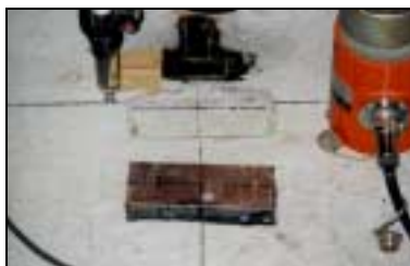
Fig. 4(c). Controlled punching shear failure of main specimen
