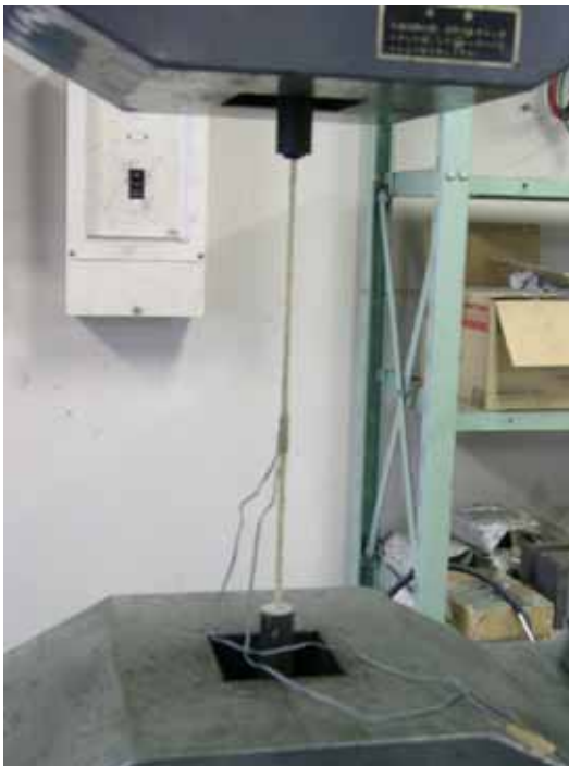
Fig.2 Tensile test of CF Rope
