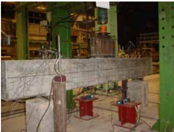
Fig.6 Test setup of loading test
