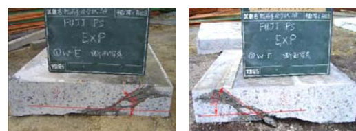
(a) Simple support Normal RC: Shear angle: 45°
