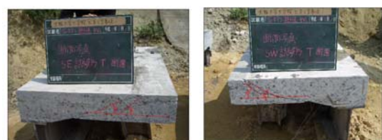
(b) Simple support Expansive: Shear angle: 35°-40°
