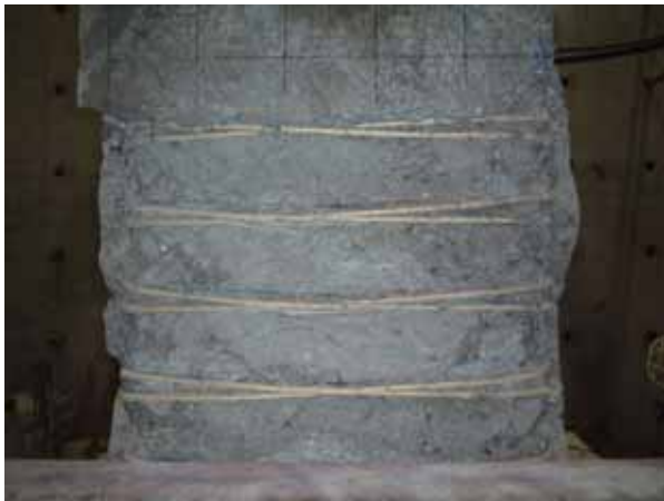
Fig.10 Failure of specimen (No.1) – jacket removed, CF Rope not ruptured
