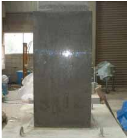
Fig.4 Jacketing for column
