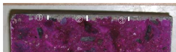
Photo 3 Measurement Points of Carbonation Depth.
