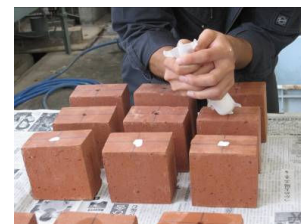
Fig. 2 Application of impregnant (water penetration barrier agent)
