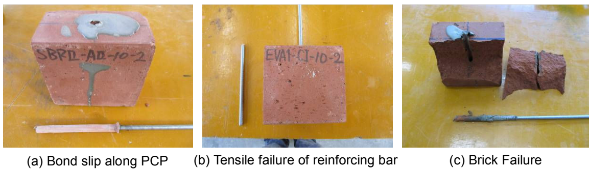
Fig. 5 Failure patterns observed during bond strength tests
