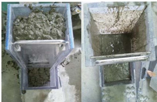
Fig.2 Fresh concrete in the room B of the U-shaped box before and after vibration
