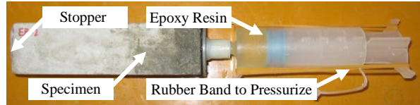
Photo 1 View of Repair Material Injection System
