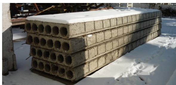
Photo 2 Precast reinforced concrete floor elements
