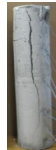
(b) Stain gauge No. and (c) Failed specimen located height (mm) 100 x 400 (W/C = 100%)
