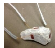
Fig. 5 Measurement of CTE of coarse aggregate
