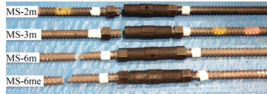
Fig.5 Failure of mechanical splices
