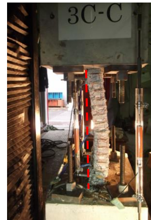
Photo 2 Final buckled shape of 3C-C specimen
