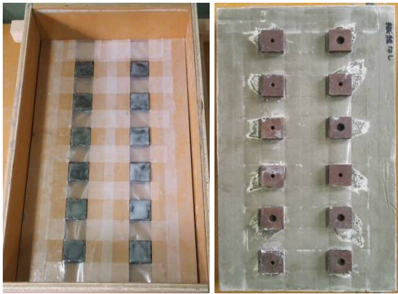
(a) 付着治具と型枠 (b) 脱型後
