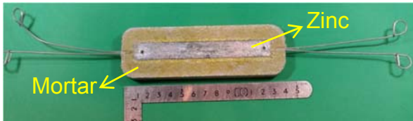
Photo 1 Sacrificial anode installed on the rebar
