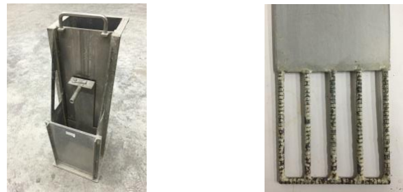
Fig.5 Concrete Box test (Left) and obstacle R1 (Right)
