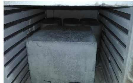
Fig.4 Concrete Specimen in an electric furnace
