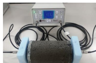
Fig. 3 Ultrasonic pulse wave velocity setup
